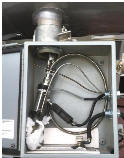
Figure 11. The Capillary and Electronics Package Were Placed in a Box with a Heater (seen at the bottom of the box) [36].
