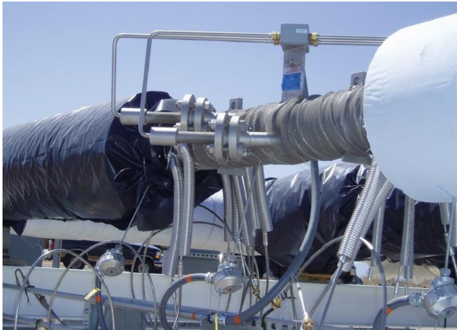
Figure 7. Flowmeter in MSTL, which remains uninsulated [36].
