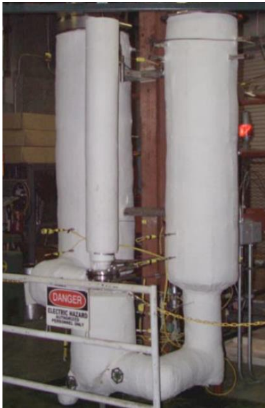
a. b. Figure 2.26. a. Thermal cycle insulated test apparatus and b. Test chamber and valving for filler materials tests [45].
