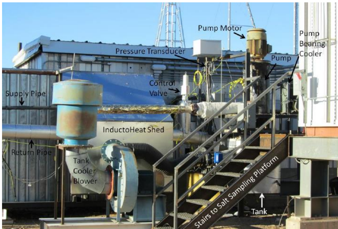
Figure 2.3. The LOFTED Pump and Test Section Installed at the NSTTF [36].
