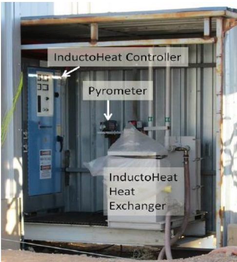
Figure 2.5. a. Electronics enclosure with InductoHeat controller, pyrometer, and heat exchanger, and b. connected cooling loop and cooler [36].
