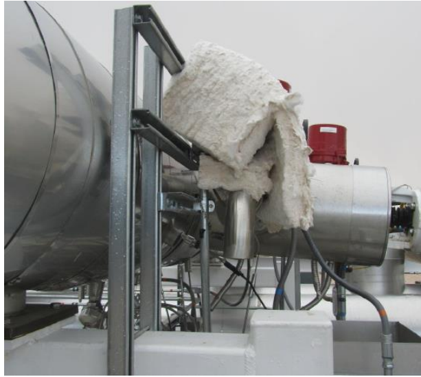
Figure 10. Test Performed by Wrapping the Box Containing the Electronics with Insulation [36].
