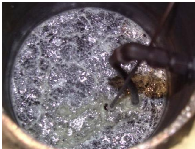
Figure 2.28. Isothermal test with typical crust formation, within the Zone 5 test pot [45].
